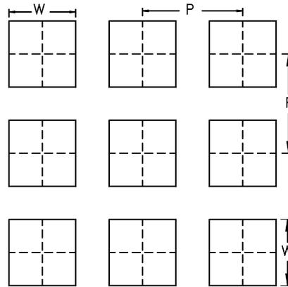
5. **Sieve Opening Size, Pitch of Openings and tolerances:** The nominal size of individual hole/aperture at mid-section (W), the Pitch of holes/apertures (P) and permissible tolerance for them shall be as under:
